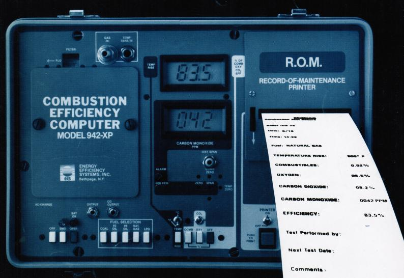
Fine tuning a furnace or boiler with the ENERAC 942-XP Combustion Efficiency Computer leaves you with something besides maximum fuel savings...
