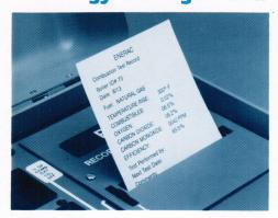
The 942-XP prints out time, date, boiler i.d. code, and all results of testing including actual combustion efficiency.
