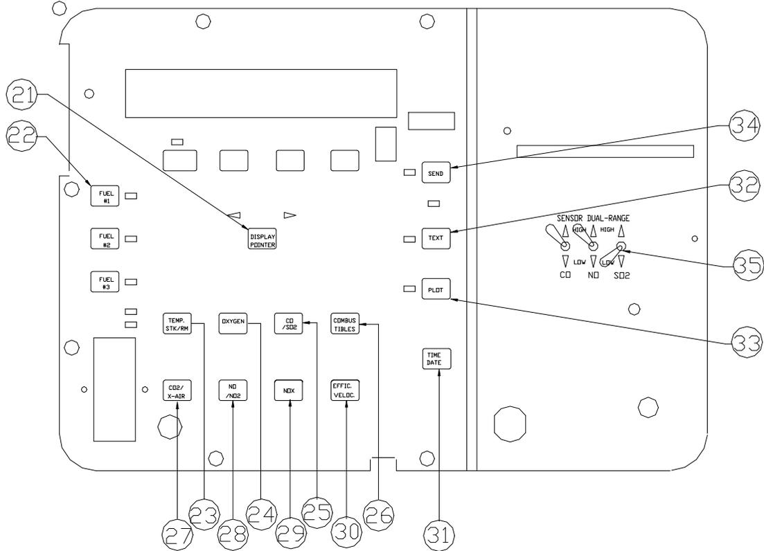
25. **CO/SO2 display key.** Press this key to display the concentration of carbon monoxide in the stack. Press it again to display the concentration of sulfur dioxide in the stack. This key toggles to display alternatively CO and SO<sub>2</sub>.
