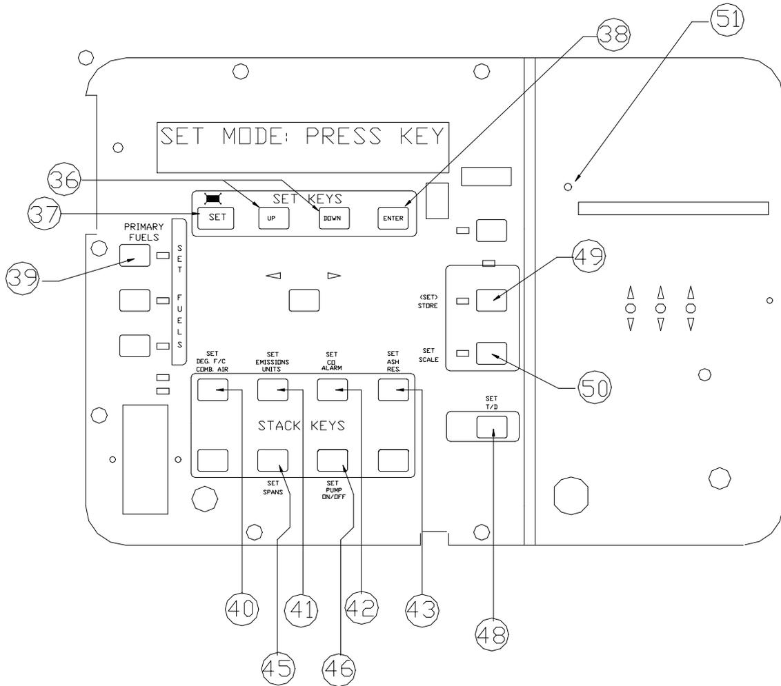
Press this key to enter the “SET” mode, (See LCD display), and change the function of the ENERAC keys to those listed outside the corresponding buttons. The LED located directly above the “SET” key will stay on as long as you are in the “SET” mode. Press this key again to exit the “SET” mode.
