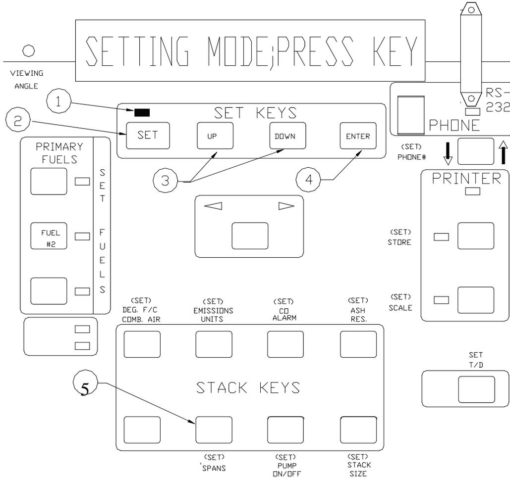
1. LED ON- "SETTING MODE";LED OFF- MEASUREMENT MODE
