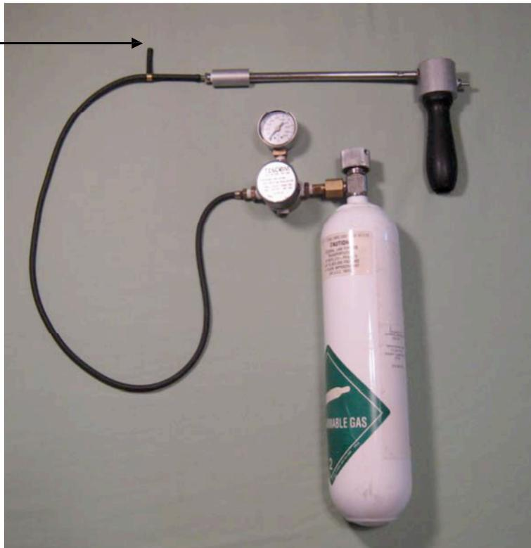
2. An optional demand-regulator will automatically supply an adequate flow of gas to the analyzer without wasting any span gas and without venting any toxic gas to your ambient environment. This accessory, shown in the figure below, is available from the factory.
