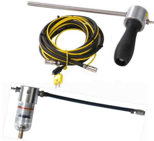
The sampling line connects to the probe and delivers the gas to the conditioning system. The hose may be made of Viton, Teflon, or EPDM. The integrated yellow wire is for connecting the thermocouple to the analyzer.
