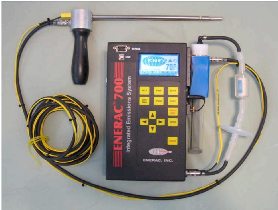
1. Remove the instrument from its case and connect the thermoelectric condenser (or water-trap) and probe to the unit.
