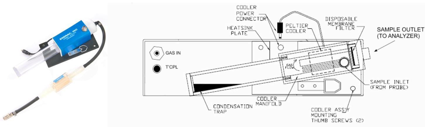
The sample, consisting of gas and partially condensed water vapor, enters the drier through the “SAMPLE INLET”. It flows through multiple narrow chilled passages, where total separation of gas and vapor occurs. The dried sample makes a 180 degree turn, flowing upwards and exiting through the “SAMPLE OUTLET”, while condensed vapor is collected in the trap.
