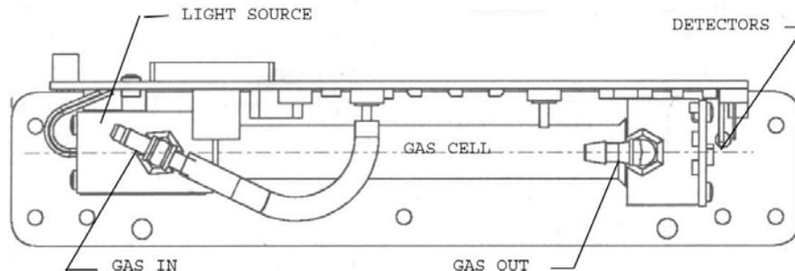
The light source is a pulsed incandescent bulb. There are four detectors: one for each gas plus a reference detector. The detectors consist of pyroelectric elements equipped with narrow-band transmission filters, each filter tuned to the absorption band of the target gas.
