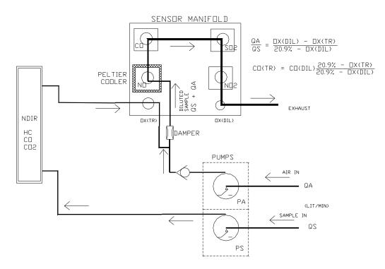
Typically the air pump has a flow rate of approximately 2,000 cc/min. The flow rate of the sample pump can be adjusted from 2,000 cc/min to 400 cc/min by reducing its duty cycle. The two oxygen sensors monitor the respective concentration of oxygen and the processor calculates the dilution ratio.
