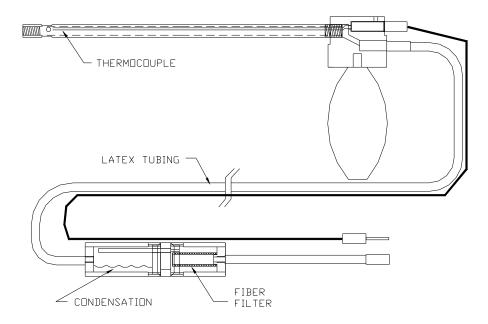
It is also recommended as a low cost option for combustion efficiency measurements. The water trap should be cleared of condensation after each use. The fiber filter should be replaced when it becomes noticeably discolored.
