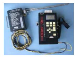
2. Make sure the instrument is in a clean-air, room-temperature environment and turn it on. If you have a problem with the display initializing, please RESET the unit.
