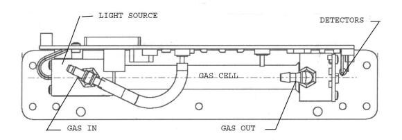
The light source is a pulsed micro bulb. There are four detectors: one for each gas plus a reference detector. The detectors consist of pyroelectric elements equipped with narrow-band transmission filters, each filter tuned to the absorption band of the target gas.
