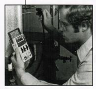
**Boilers and furnaces:** ENERAC Pocket 60 comes with a 10" stainless steel probe and is calibrated to provide accurate readings in both high and low temperature applications.
