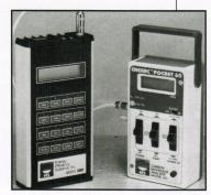
24 Hour Monitoring: These units can be equipped with a data output that can be used for unmanned around the clock measurements of gas emission in boilers, furnaces, and ambient air.
