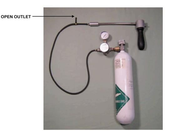
2. <u>An optional demand-regulator</u> will automatically supply an adequate flow of gas to the analyzer without wasting any span gas and without venting any toxic gas to your ambient environment. This accessory, shown in the figure below, is available from the factory.
