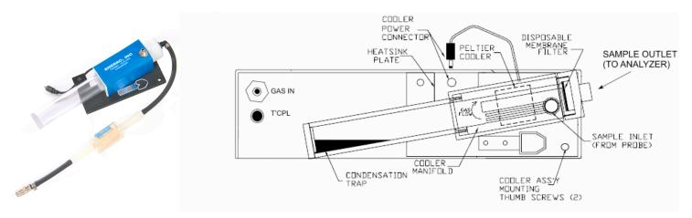
The sample, consisting of gas and partially condensed water vapor, enters the drier through the "SAMPLE INLET". It flows through multiple narrow chilled passages, where total separation of gas and vapor occurs. The dried sample makes a 180 degree turn, flowing upwards and exiting through the "SAMPLE OUTLET", while condensed vapor is collected in the trap.
