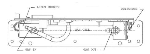
The light source is a pulsed incandescent bulb. There are four detectors: one for each gas plus a reference detector. The detectors consist of pyroelectric elements equipped with narrow-band transmission filters, each filter tuned to the absorption band of the target gas.
