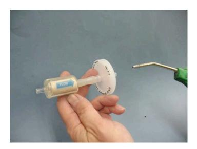
An additional membrane filter, if present, is located inside the thermocooler's white plastic cap.
